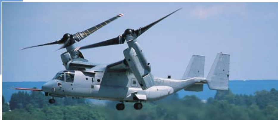
V-22 TILTROTOR can ascend vertically, with its proprotors pointing straight up. An alternative, shown here, is a short takeoff mode, which enables the craft to be more heavily loaded. In this mode the proprotors are tilted forward, providing some horizontal thrust.
