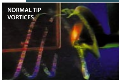
CAVITATION OCCURS ON LOW-PRESSURE SURFACE
