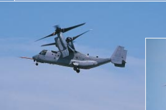
V-22 TILTROTOR can ascend vertically, with its proprotors pointing straight up. An alternative, shown here, is a short takeoff mode, which enables the craft to be more heavily loaded. In this mode the proprotors are tilted forward, providing some horizontal thrust.
